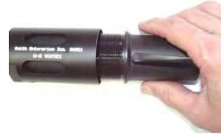
15. Note how the edge of the Coupler extends ever so slightly over the **VORTEX**<sup>®</sup> Flashhider. At this point of the installation, there should be no wobble, lateral or forward-backward movement of any kind of the **VORTEX**<sup>®</sup> Flashhider assembly on the end of the barrel.
