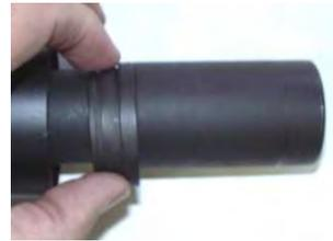
9. Gently pull the O-Ring forward towards the muzzle and fit over the Half Rings and seat the O-Ring into the groove in the split rings.
