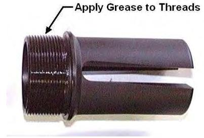
14. Screw the **VORTEX**<sup>®</sup> Flashhider into the Coupler by hand as far as it will go. The flats on the Coupler are 1- 3/4 inches across the wrench flats. Use a wrench or strap wrench on the Coupler and a rod or anything else that is no more than 1/4 inch thick on the Flashhider placed between the prongs at the base (thread end) and tighten.
