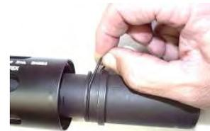
10. The O-Ring will fit flush in the groove.
