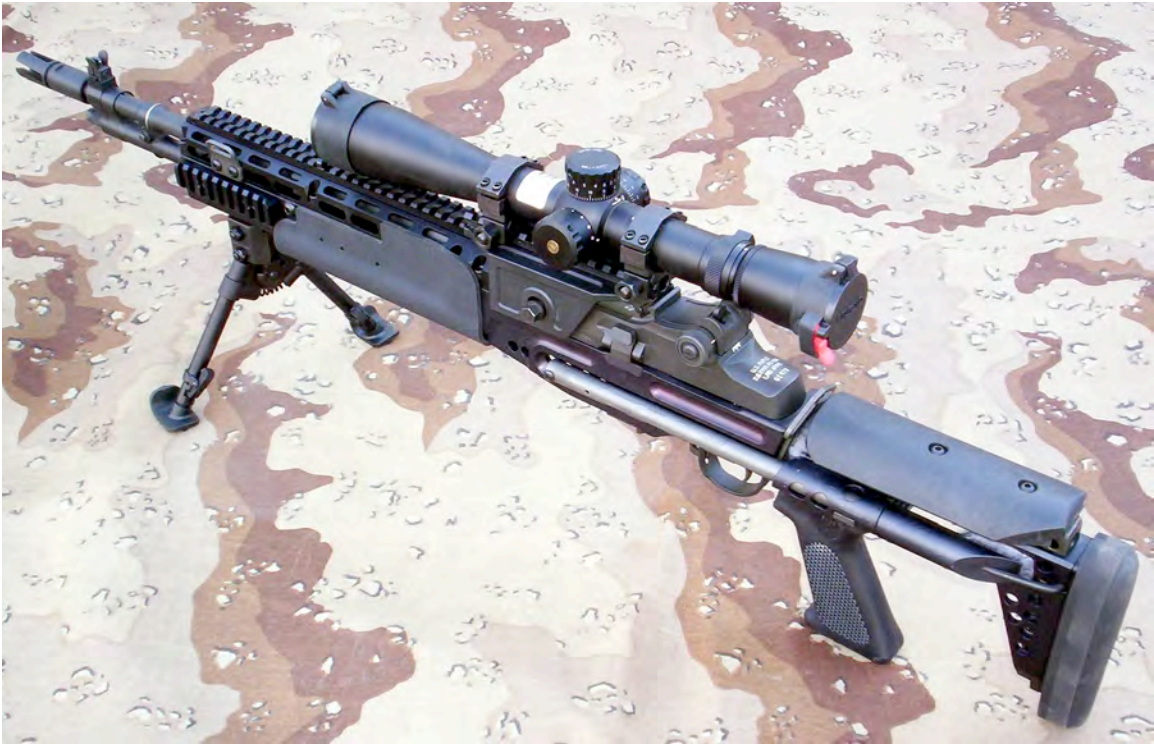
Fig. 2 Lightweight QD MIL STD 1913 Bipod fitted to MK14 Mod SEI Rifle.
